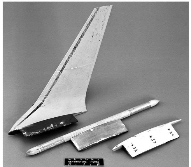
Fig. 3 Wing-tip configurations tested: winglet, pencil tip store, and clean wing tip.
